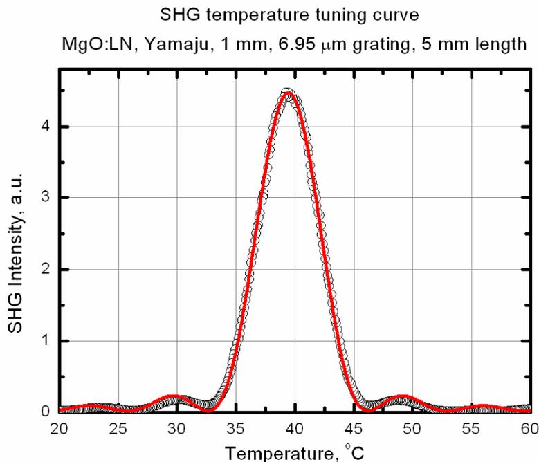
**Fig. 7.** Temperature dependence of the green light maximum intensity (532 nm output power) for MgO PPLN period 6.95 microns. The dots are experimental data and the solid curve is theoretical curve for a 5 mm length.
