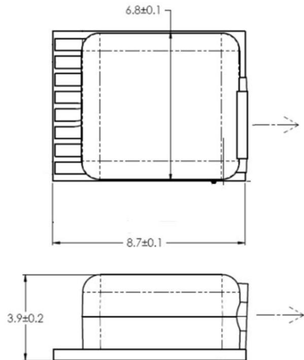
Figure 2. Drawing of ATTO-K miniature laser package developed by Spectralus
