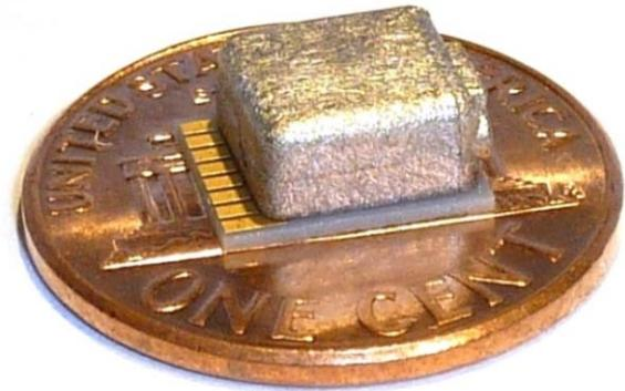
Figure 1. ATTO-K miniature laser package developed by Spectralus pictured on one US cent coin
